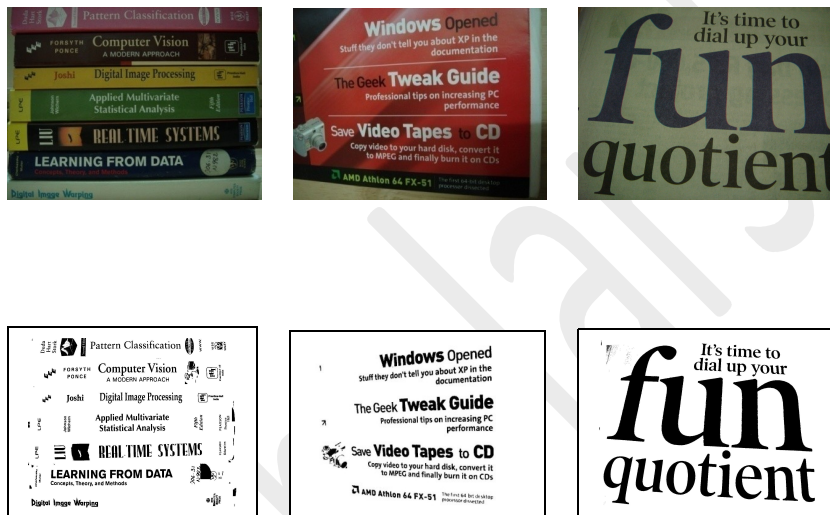
Fig. 1. Some example outputs of binarization. As desired, the output binary images have black text on a white background irrespective of their colors in the input images.
